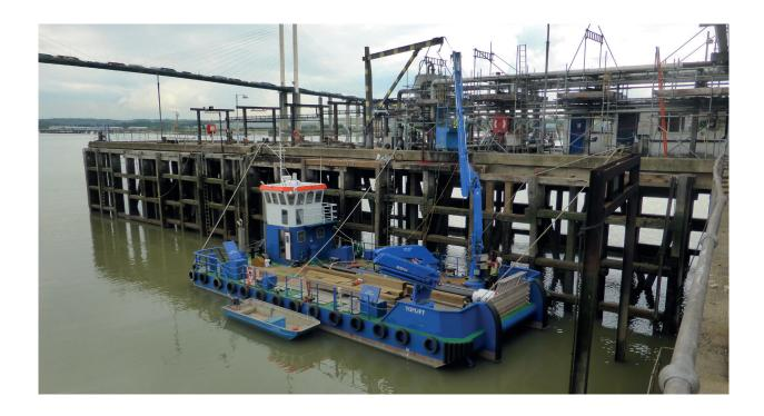
**TOPLIFT** is a multicat workboat with multi-purpose capability offering large deck cargo capacity, twin deck cranes, shallow draft, fresh water and fuel cargo tanks, spud legs and winch capability. Classed to MCA Category 2 (60 nautical miles from a safe haven) Vessel hull can be separated for road transportation.
